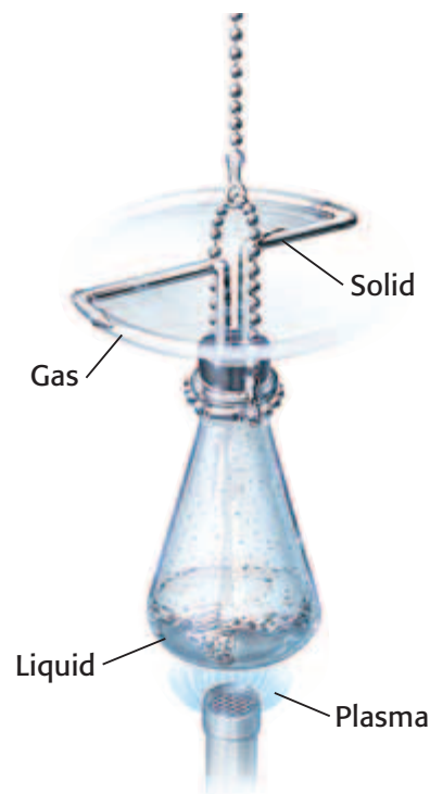
Figure 1 This model of Hero's steam engine spins as steam escapes through the nozzles.
